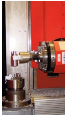
NC gripper loading the part into the lathe spindle
