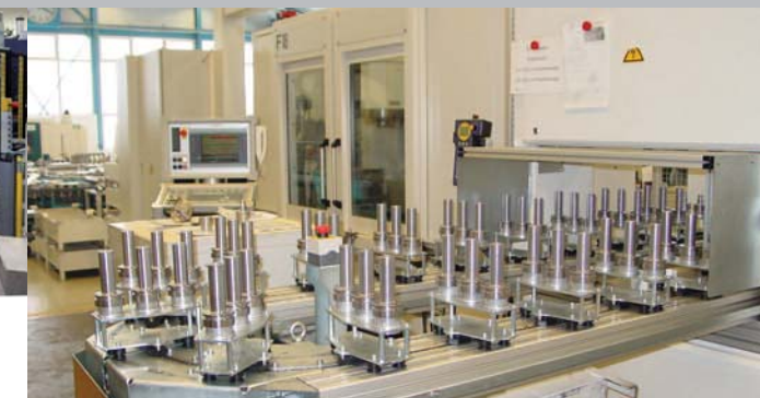
Magazing and loading of chucks by gantry loader
