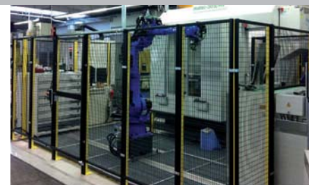
Robot loading of drawer magazines
