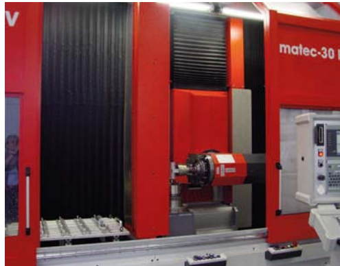
Pendulum machining. Workpiece handling by means of an NC gripper, loaded from the tool magazine. Working area on the left side: Raw parts/finished parts Working area on the right side: machining
