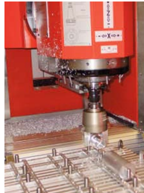
NC gripper depositing the part
