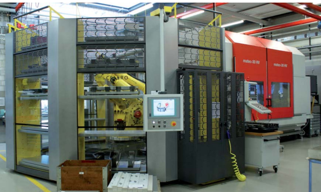
Gantry loader, pallet magazine or robot loading
