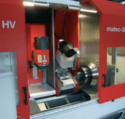
matec-30 HV with bar feeder and saw unit for machining from the bar
